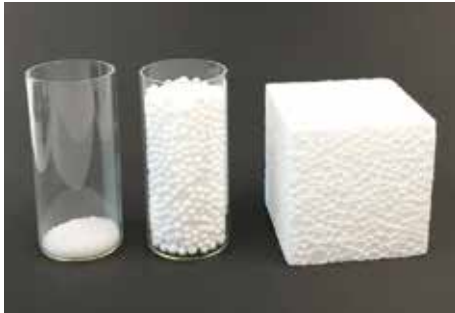
Up to now, steam has been used for prefoaming of EPS microbeads (left) and fusion of the foamed beads (center, same mass) to yield the EPS molded part (© NMB)
