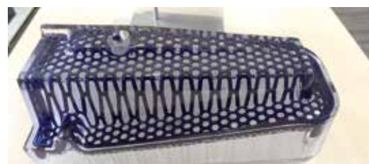
Plastic model of a 3D-printed variothermal mold. The branched runner network of the surface tempering system is shown in blue. This enables the cavity surface to be heated or cooled down to the process temperature within seconds (© Hofmann)
